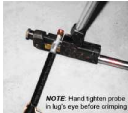
Figure A2.13. Crimping Compression Lug.
