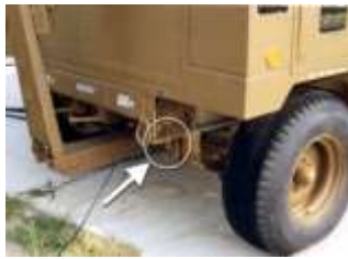
Figure 5.7. Ground Stud on MEP-12A Generator.
