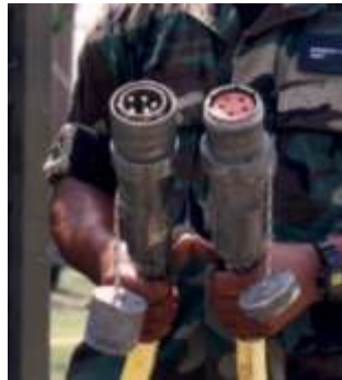
Figure 2.15. Low-Voltage Cables with Cannon Plug Connections.
