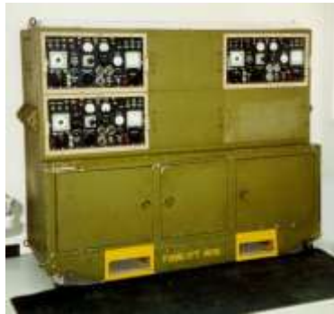
Figure 2.17. Equipment Rack with Generator Control Panels.
