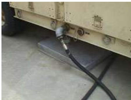
Figure 5.10. Fuel Hose Connected to MEP-12A.
