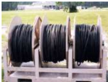
Figure 2.7. Cable Reel Pallet Assembly (CRPA).
