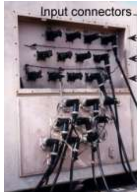
Figure 5.23. PDC Line Side Connection.
