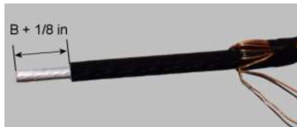
Figure A2.12. Insulation and Conductor Shield Removed.
