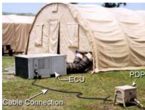
Figure 4.19. Connection from PDP to ECU.
