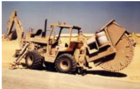
Figure 4.7. Tractor with Backhoe, Blade, and Trenching Wheel.
